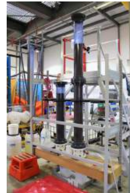
1m and 2m Heap Leach Columns at ANSTO
