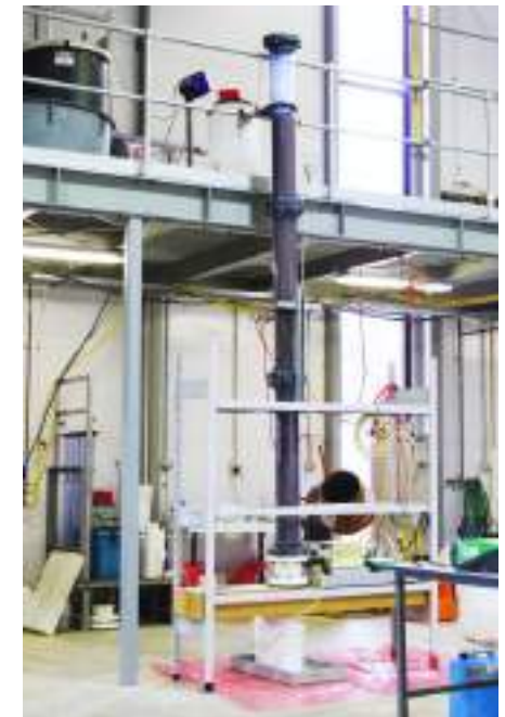
3m Heap Leach Columns at ANSTO
