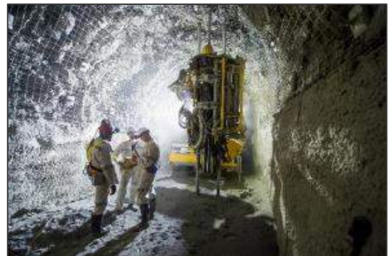
Long hole drilling
