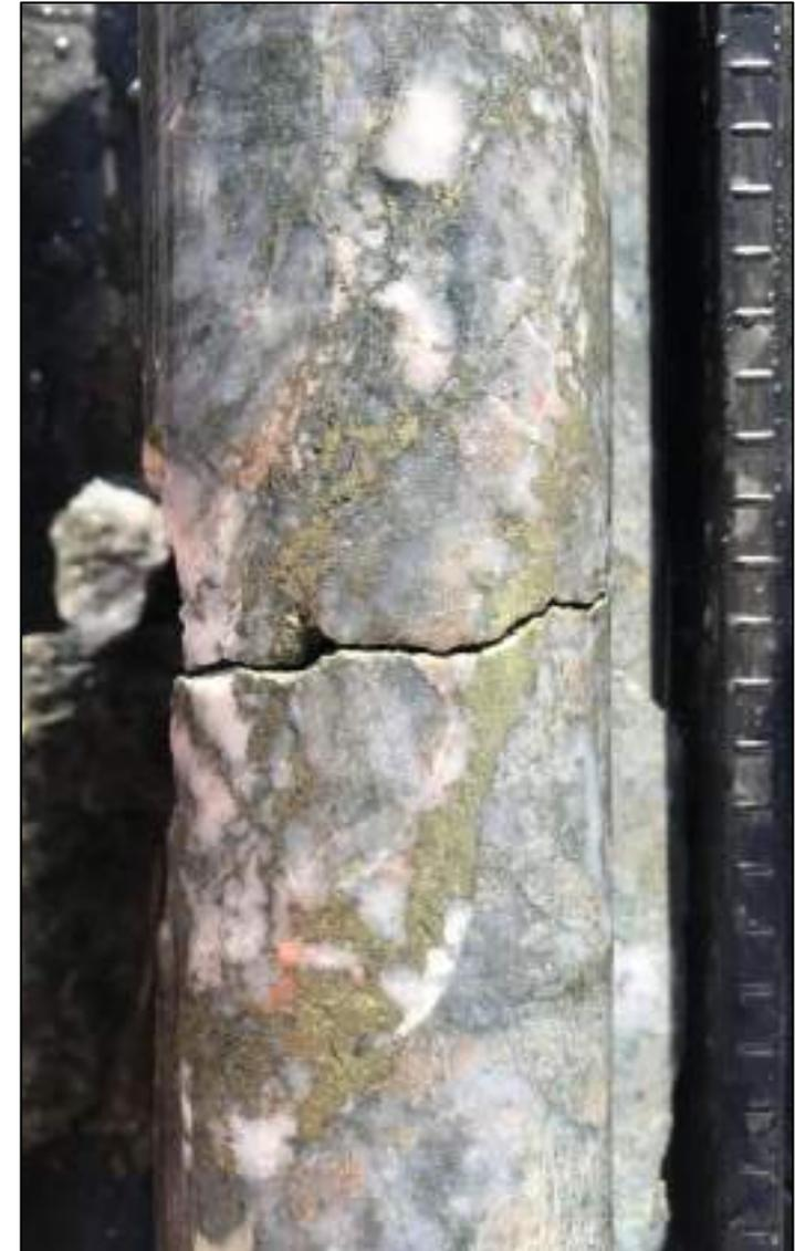
Chalcopyrite from the breccia intersection in AND005 from HQ core drilling at Anagulu Prospect
