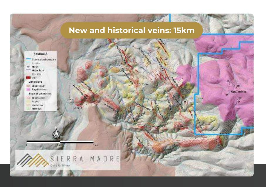
An overly complex structural interpretation with inferred faults guided previous drilling and assumed the Dos Hornos breccia veins were cut off.
