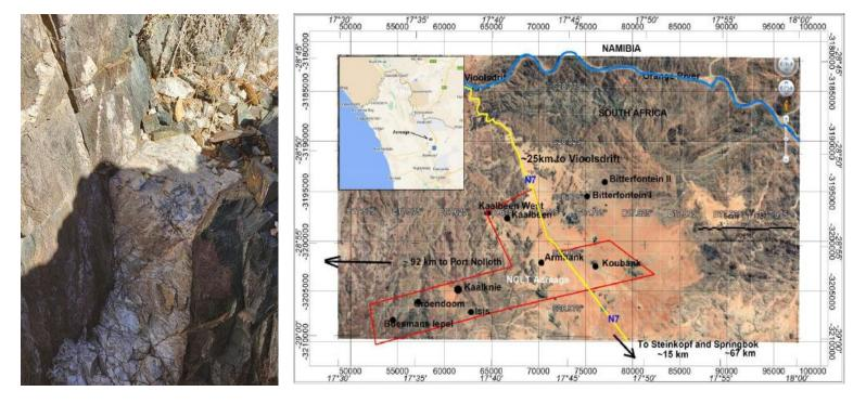
**Fig 1:** Ore vein of 0.6m width in main excavation
