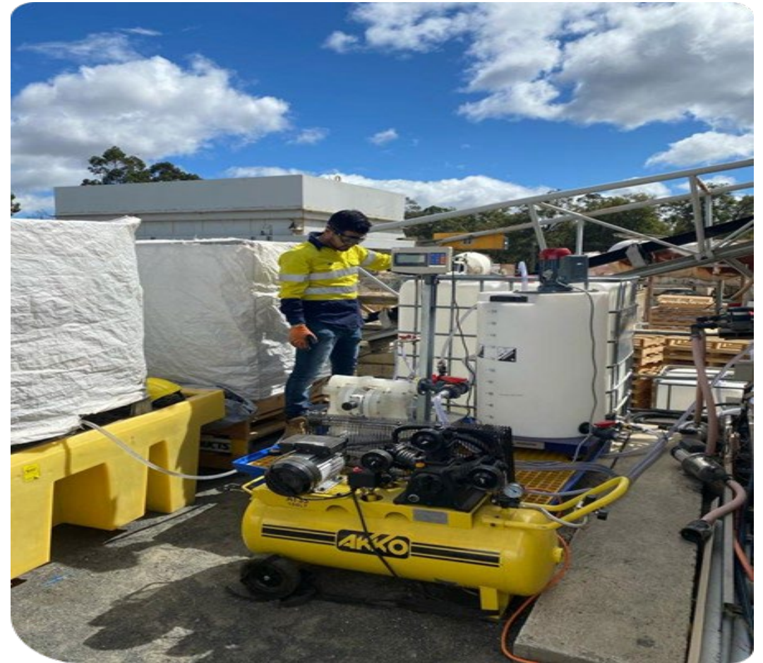
Figure 1: Geopolymer Pilot Batching Plant
