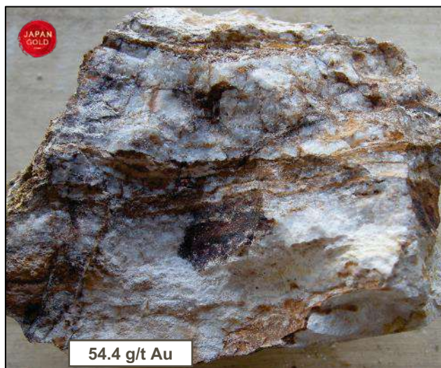
Kitano-o Mine sample: Banded quartz vein collected from dump material of underground working in central Kitano-o; JG0069: 54.4 g/t Au, 7 g/t Ag
