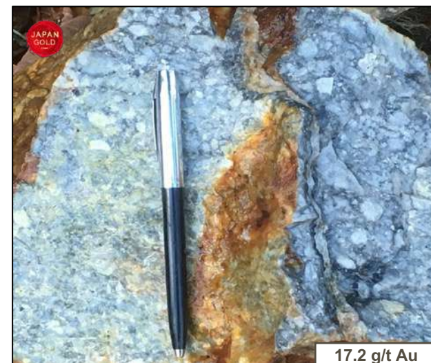
Sakinzawa Workings sample: gold-bearing quartz stockwork in rhyolitic breccia outcrop; SAM02069: 17.2 g/t Au, 16 g/t Ag
