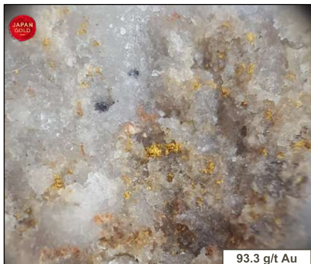
Showa Mine sample: visible gold in quartz stockworks cutting silicified laminated mudstone, field of view is approximately 1 cm; SAM01867: 93.3 g/t Au, 17 g/t Ag
