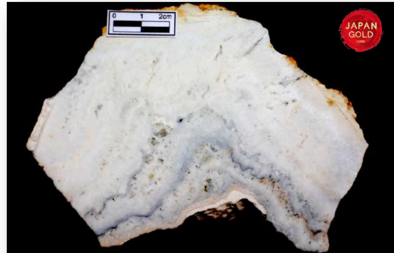
Ginguro banded quartz vein. Collected from the Kitano-o Prospect located in the Ikutahara Project . 60.8 g/t Au and 89.6 g/t Ag.
