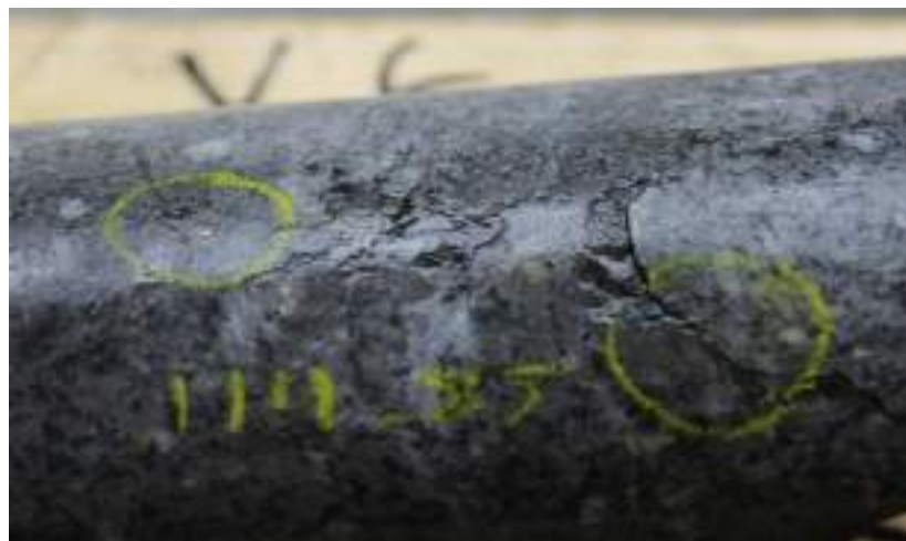
Visible Gold Core Samples From the Host Rock Granodiorite in the Central Zone
