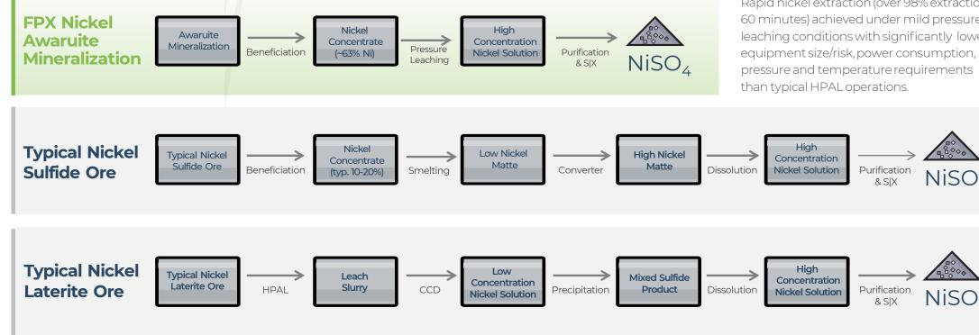
Baptiste's Awaruite mineralization promotes a simple 3-stage process with the potential to be more efficient than the typical 5-stage processes required to convert sulphide and laterite ores into nickel sulphate.
