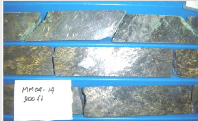
Above: Drill core from MM04-14 at Makwa averaged 1.74% Ni, 0.12% Cu, 1.81 g/t Pd, 0.45 g/t Pt 0.026% Co over 16.5m under the resource pit shell ( apparent width )
