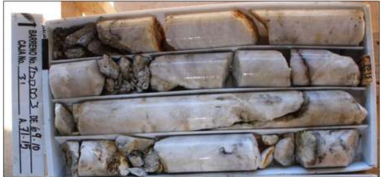
Figure 5. TDD-003 at 69m: Banded chalcadonic quartz vein and breccia
