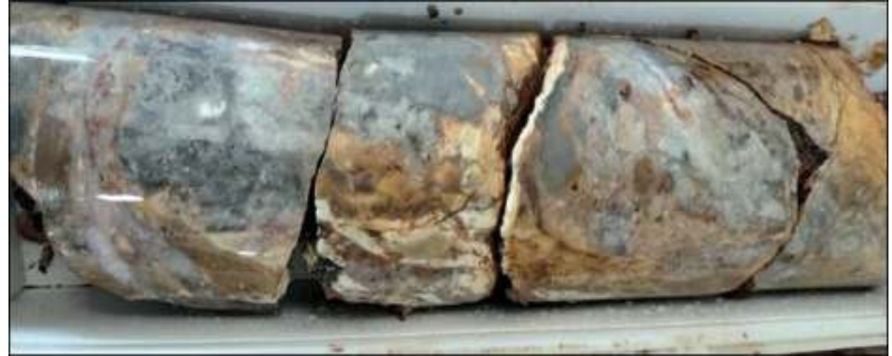
Figure 5. TDD-003 at 69m: Banded chalcadonic quartz vein and breccia
